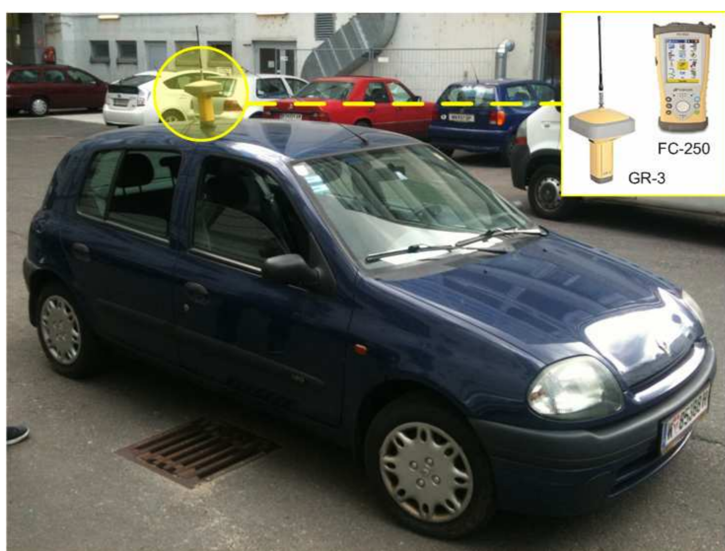
Fig. 1: Measurement system consisting from Topcon GR-3 receiver [1], FC-250 field controller [2] and moving vehicle
